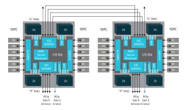
Figure 7: EPYC 9005 Series processors in a 2-socket configurations
