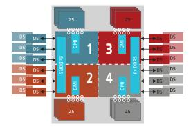
Figure 8: Dividing an EPYC 9005 Series processor into four NUMA domains can give small performance improvements for some applications
